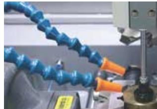
Air cooling system
