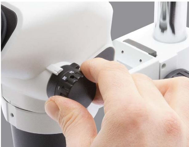
Coarse and fine focusing knobs
