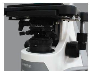
X-LED Full Koehler type transmitted illumination
