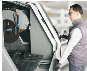
Two Hand Control For Safety Operation
