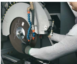
Easy Exchange of Cut Off Wheel
