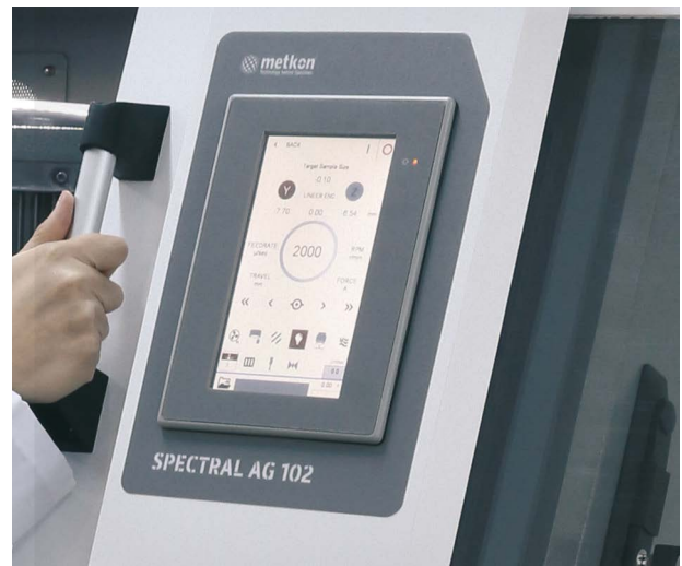
HMI touch screen controls with various grinding methods and database with grinding programs and maintenance monitoring
