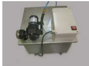
Recirculating Coolant System
