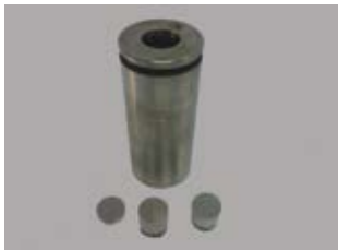
Mould assembly, with intermediate ram
