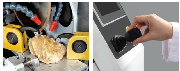
GEOCUT 302-S is a robust manual cutter with X-Y bed designed for cutting minerals, rocks, concrete, glass, ceramics, refractory and other geological samples
