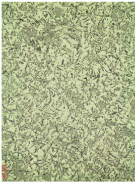
Etial 160 Aluminum Magnification: 100 x
